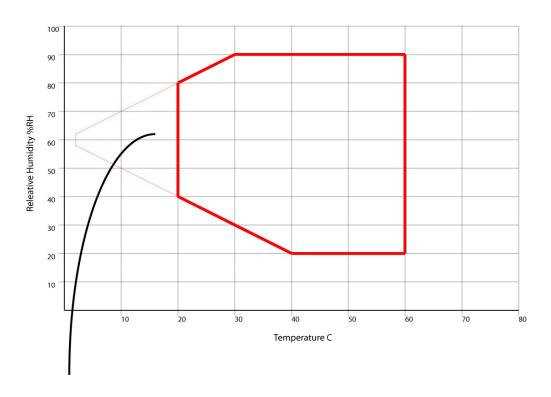
If the temperature setpoint is below 20 or above 80C, the RH control will be disabled and the chamber will adopt a natural value depending on the internal chamber conditions
