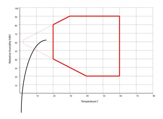
If the temperature setpoint is below 20 or above 80C, the RH control will be disabled and the chamber will adopt a natural value depending on the internal chamber conditions
