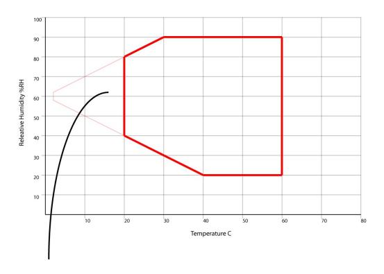
If the temperature setpoint is below 20 C, the RH control will be disabled and the chamber will adopt a natural value depending on the internal chamber conditions
