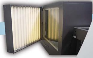
The powerful air circulation fan is also used to drive air over a waterbath whose temperature is accurately controlled by a precision RH sensor and an environmentally friendly CFC-free refrigeration system. This results in extremely stable humidity control between 10% and 90% RH. Various lighting options are available, from basic ON/OFF control to stepless intensity control at any value between 10% to 100%.
